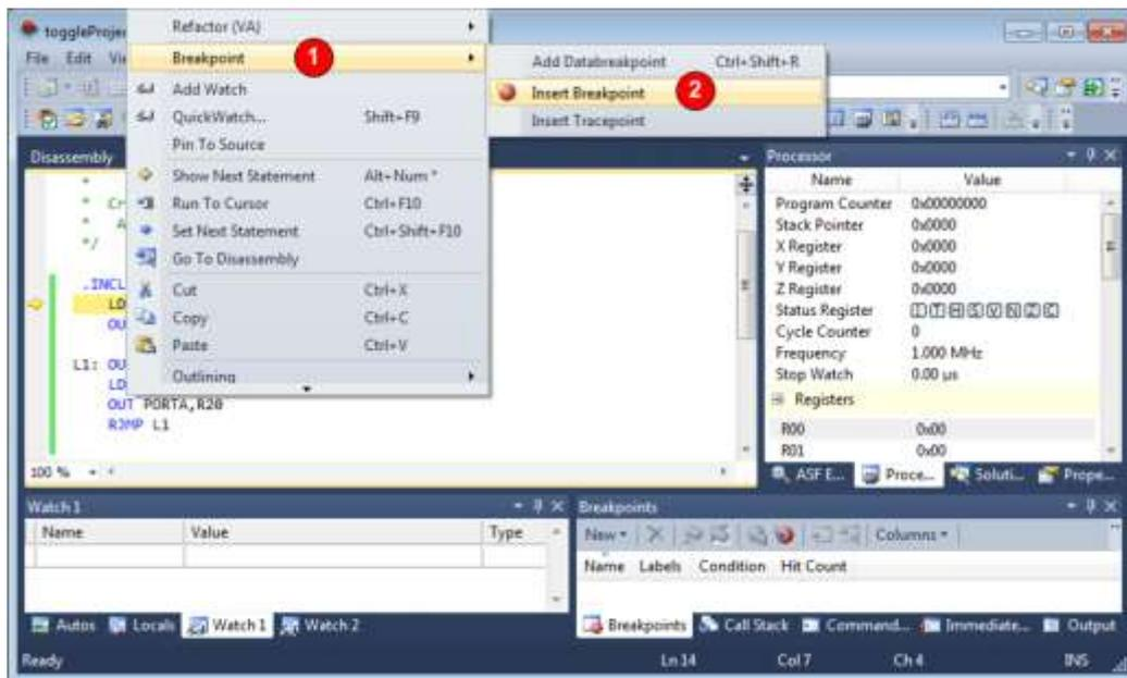
2. Press **F5** or the **Run** button. The IDE runs program until it reaches the Breakpoint. Now, you can continue debugging from the breakpoint using the **Step into** and **Step over** buttons.
