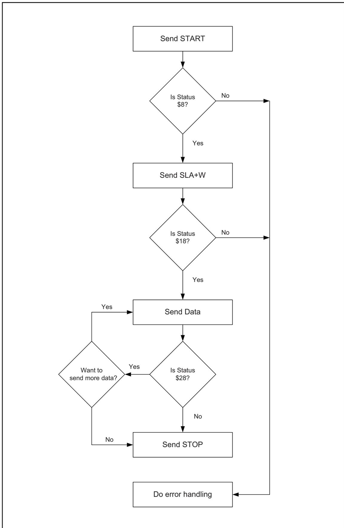
Figure 18-18. Programming Steps of Master Transmitter Mode with Checking of Flags
