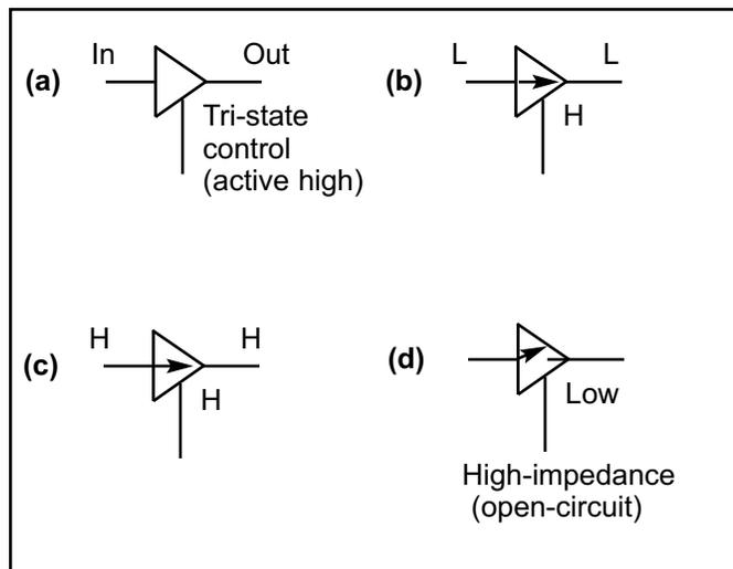
**Figure C-9. Tri-State Buffer**
