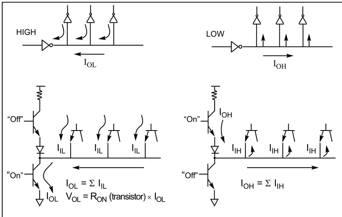
**Figure C-7. Current Sinking and Sourcing in TTL**
