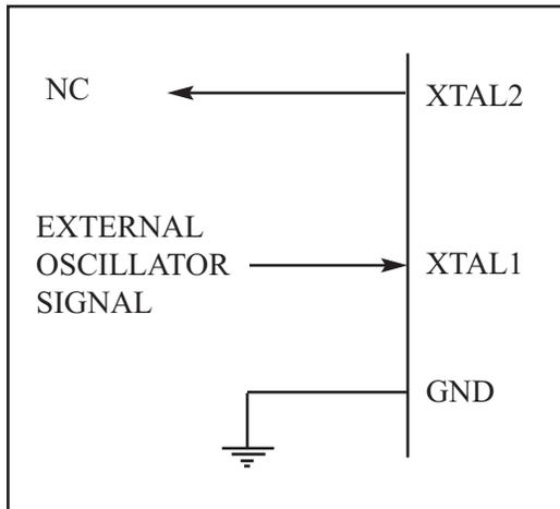
**Figure 8-6a. XTAL1 Connection to an External Clock Source**
